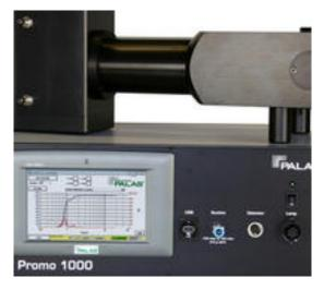
The success of the Palas<sup>®</sup> aerosol spectrometers is based on the development of а measurement method with white light source, 90° scattered-light detections and а measurement volume that was defined optically by the University of Karlsruhe, KIT.
